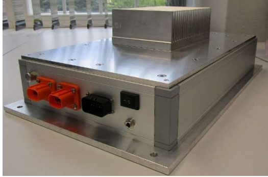
Figure 5: Automotive-compliant prototype of the developed DC/DC converter for LadePV
