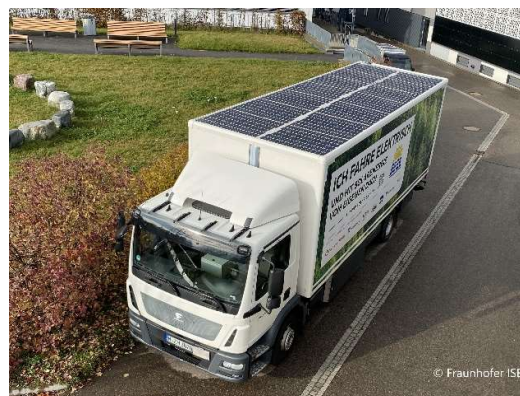
Figure 1: Demonstrator truck with integrated photovoltaic modules in the roof
