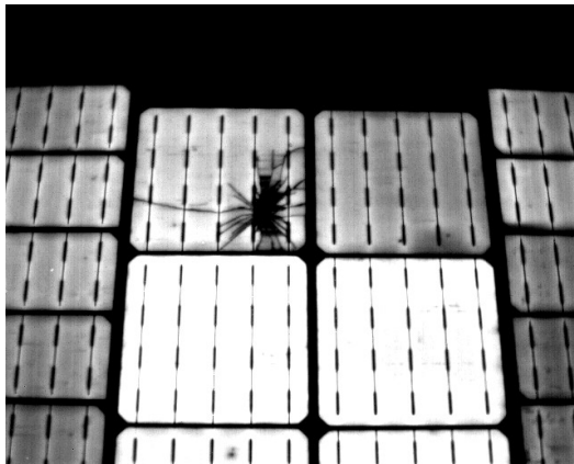
Figure 9 Close-up of EL measurement to a damaged PV module on the solar roof taken by a daylight EL camera.
